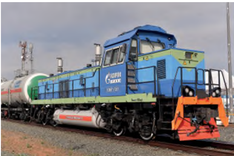
Gas-piston maneuvering locomotive TEMG1 in the Orenburg region
