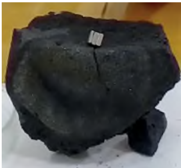
Massive superconducting bismuth cuprate synthesized in the Large Solar Furnace (Parkent) and its submicron layered structure
