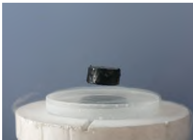
Expulsion of a superconductor by a magnetic field
