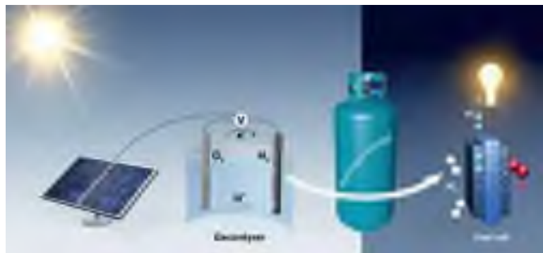
Obtaining hydrogen from water using solar energy
