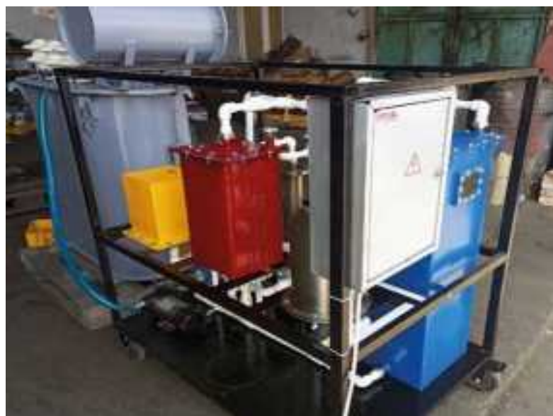
Processes of purification of used transformer oils at the Zartransformator LLC enterprise using a developed domestic mobile device (Patent of the Republic of Uzbekistan No. FAP 02334).
